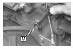
Figure 2-9: Gear oil level check plug.
